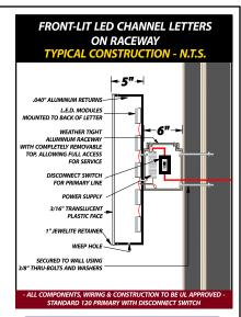
This sign is intended to be installed in accordance with the requirements of Article 600 of the National Electrical Code and/or other applicable local codes. This includes proper grounding and bonding of the sign.
