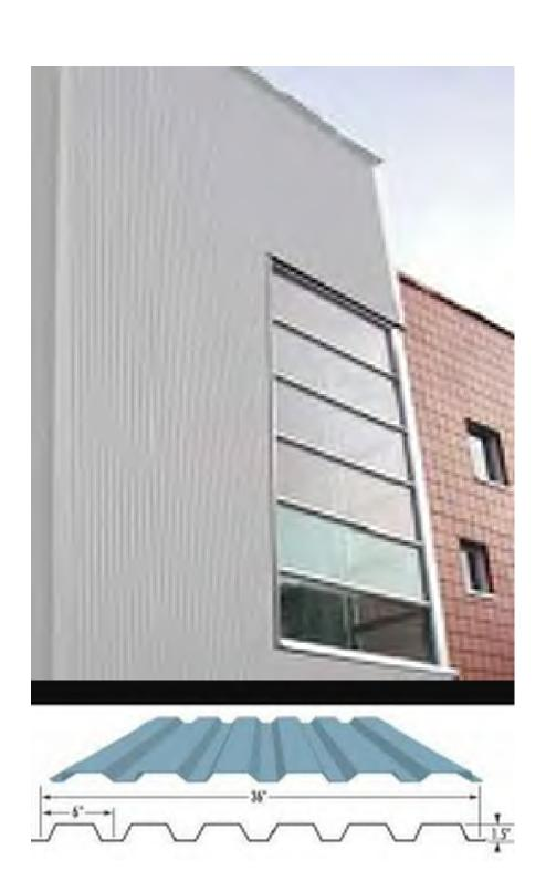
CORRUGATED METAL: SHOP PTD. KYNAR FINISH PPG COLOR "GRAY SPARKLE" UC125548 OR ALTERNATE MANUF. EQUIVALENT. NOTE: ALUMINUM PARAPET COPING TO BE SHOP PTD. TO MATCH.
